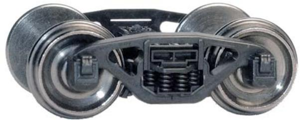
Many freight cars built in the 1920s were equipped with Dalman trucks. The Dalman 2-level truck design used additional springs to give a smoother ride. Railroads using this version include Chesapeake and Ohio, Chicago Great Western, Illinois Terminal, L&N, Milwaukee Road, M-K-T, Nashville Chattanooga and St.Louis, Pere Marquette, and many Texaco 10,000 gallon tank cars.
